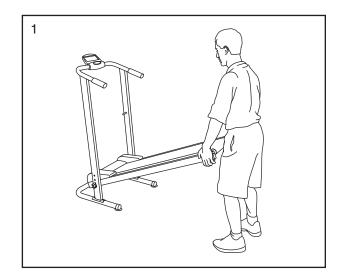
2. Hold the treadmill securely with your left hand as shown. Insert a Pin (4) into the hole in the right side of the Right Upright (36) and into the Frame (29) as far as it will go.
